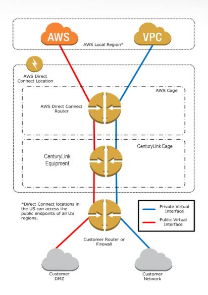
AWS Direct Connect links your internal network to an AWS Direct Connect location.
